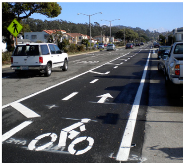
The use of pavement markings delineates space for bicyclists to ride in a comfortable facility.
