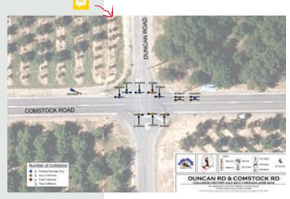
The project enhances safety for motorists by replacing the partial stop-controlled intersection with a roundabout, thereby providing better traffic operations and reducing the number of conflicting movements. A key concern along this corridor was speed and sight distance at the intersection. This project offers a form of traffic calming by reducing speeds and with the additional lighting improves visibility for motorists entering the intersection.
