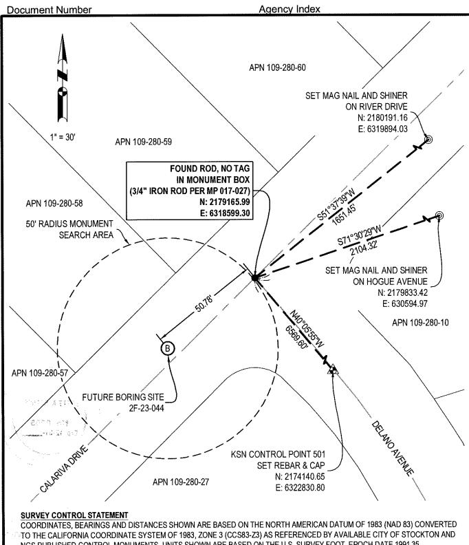
NGS PUBLISHED CONTROL MONUMENTS. UNITS SHOWN ARE BASED ON THE U.S. SURVEY FOOT, EPOCH DATE 1991.35 ADJUSTMENT, ALL COORDINATES AND DISTANCES ARE GRID, TO CONVERT GRID DISTANCES TO GROUND, MULTIPLY BY 1,00005972, THE CONVERGENCE ANGLE IS -0°30'26". THE CSF WAS DETERMINED AT CONTROL POINT 501.
