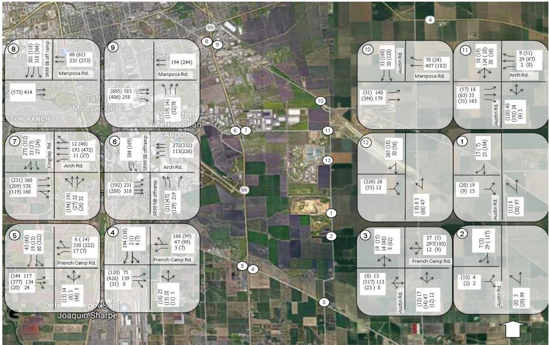
Figure 3 Existing (2018) Study Intersection Peak-hour Traffic Volumes Forward Landfill Traffic Study
